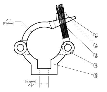
Total Width (with wing nut): 2.1" [53.2mm] Total Height: 2.1"[53.2mm]
